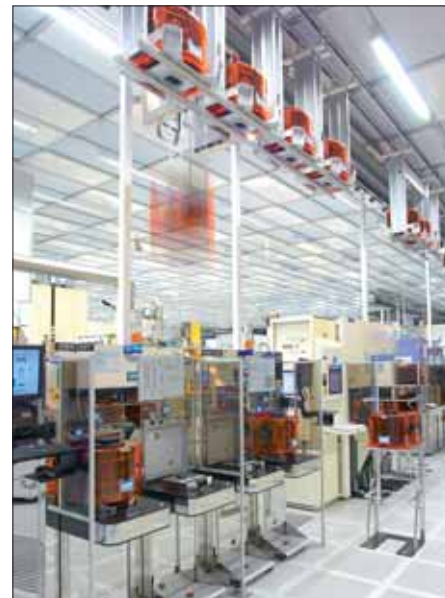
300mm Crolles clean room and the Automatic Material Handling System
