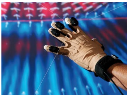
Force and tactile feedback from seismic data on a haptic virtual workstation
